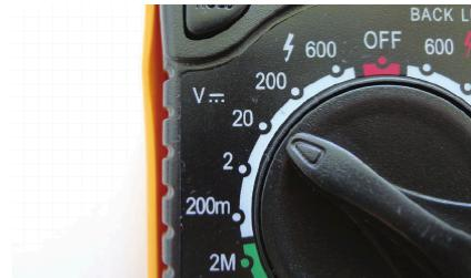
The multimeter knob set to measure voltage
