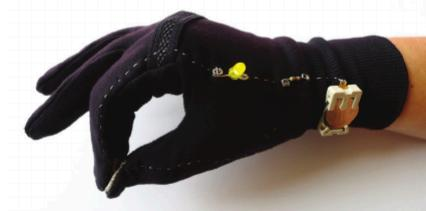
Glove with contact switch closed
