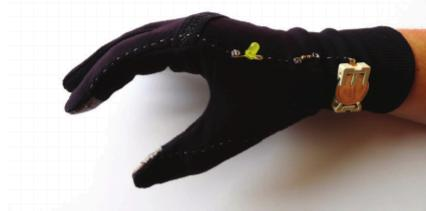
Glove with contact switch open
