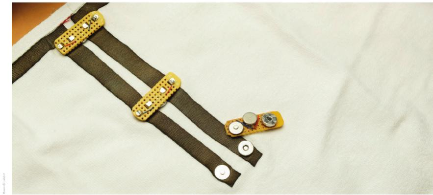
*The combination of protoboard and magnetic snaps can be used to create components that are easy to remove when the garment needs to be washed.*
