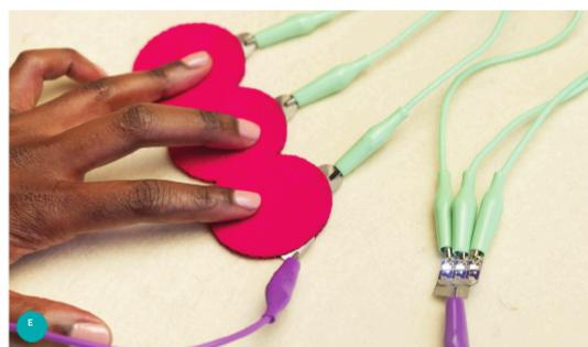
**HOW TO: Multiple DIY Pressure Sensors**
