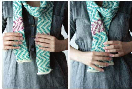
A contact switch created by *Erin Lewis* integrates conductive thread with knitted yarn: When the pink patches of the scarf are held together the switch is closed.
