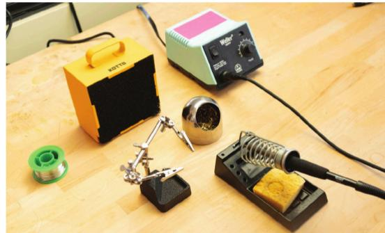
Tools for soldering: solder, fume extractor, helping
