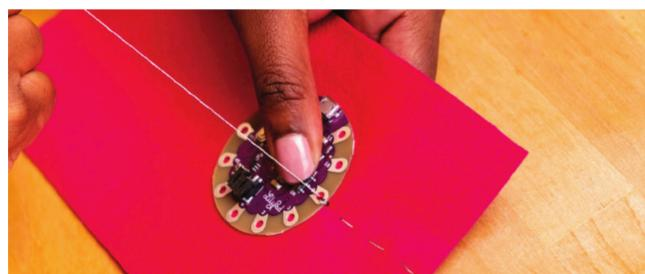
*When sewing a sew tab with conductive thread, be sure to pull the thread all the way through.*
