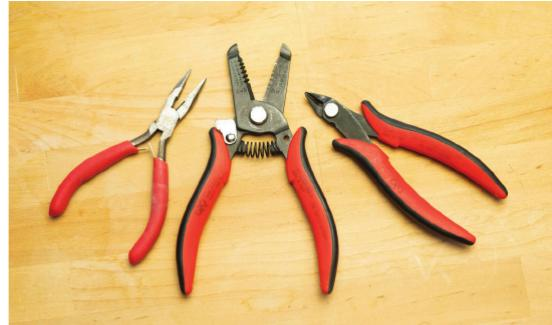
Tools for working with wire: needle-nose pliers,
