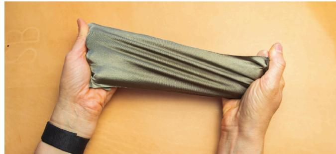
*Stretch conductive fabric is slightly more difficult to work with but works well with bendy parts of the body.*
