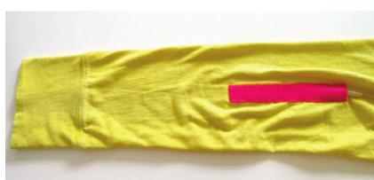
A fabric pocket is added to the sleeve to hold flex sensor in place.
