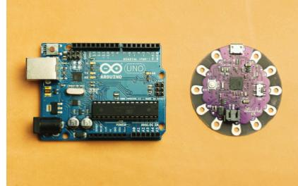
Arduino Uno (left) and LilyPad Arduino USB (right)
