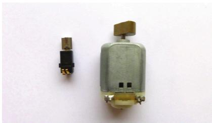
Vibrating motors with exposed heads
