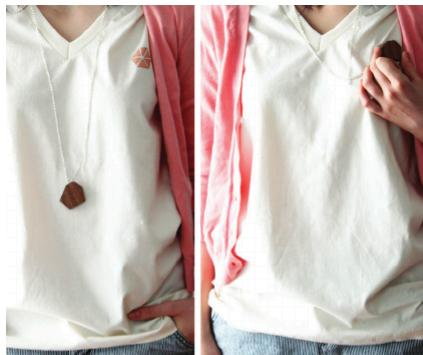
This T-shirt-and-necklace pair, designed by Jackson McConnell, uses conductive fabric on the back of a pendant to bridge the conductive-fabric pieces on the chest of the T-shirt.
