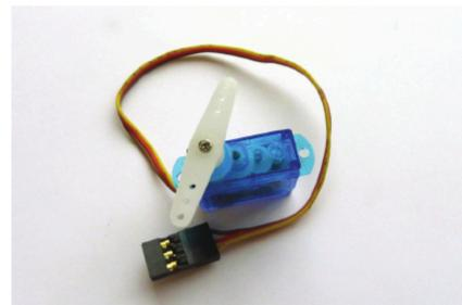
Small servo with propeller attached
