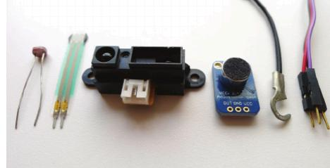
*Sensors with different connectors—left to right: legs, terminals, JST connector, pins, hook, male headers*
