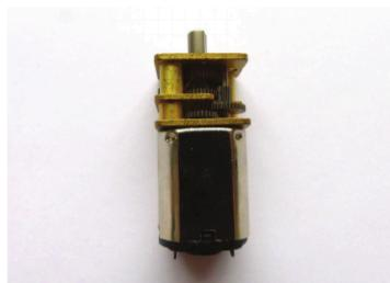
Close up of a very small gearhead motor
