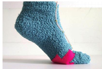
When pressure is applied to the ball of the foot, the microcontroller can read the change in sensor data.
