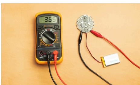
Measuring voltage from VOut pin as 3.65 V
