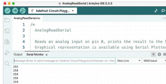
*Light-sensor values as seen in the Serial Monitor*
