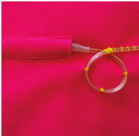
*This secured loop of wire provides strain relief
