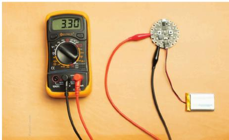
Measuring voltage from 3.3V pin as 3.30 V when CPX is powered via 3.7V lithium polymer (LiPo) battery. Note that this voltage passes through a 3.3V regulator rather than being the raw voltage from the power source.
