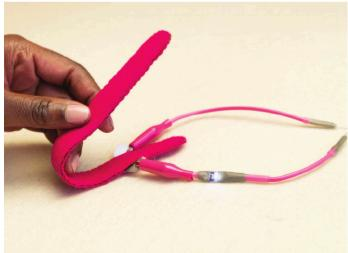
This technique can also be used to create DIY flex sensors.
