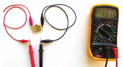
The voltage reading for a used CR2032
