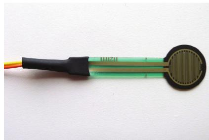
Heat-shrink tubing is used to protect the delicate solder connections between the sensor and wires.
