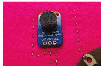
Holes meant for headers can also be used for conductive-thread connection.
