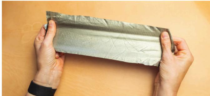
*Ripstop conductive fabric does not stretch and is very easy to sew.*
