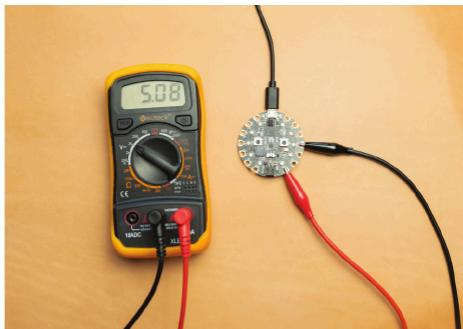
Measuring voltage from VOut pin as 5.08 V
