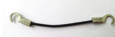
Stretch sensors with hooks attached
