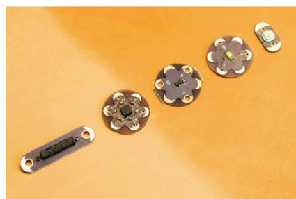
*LilyPad Reed Switch, accelerometec temperature sensor, light sensor, and push button*
