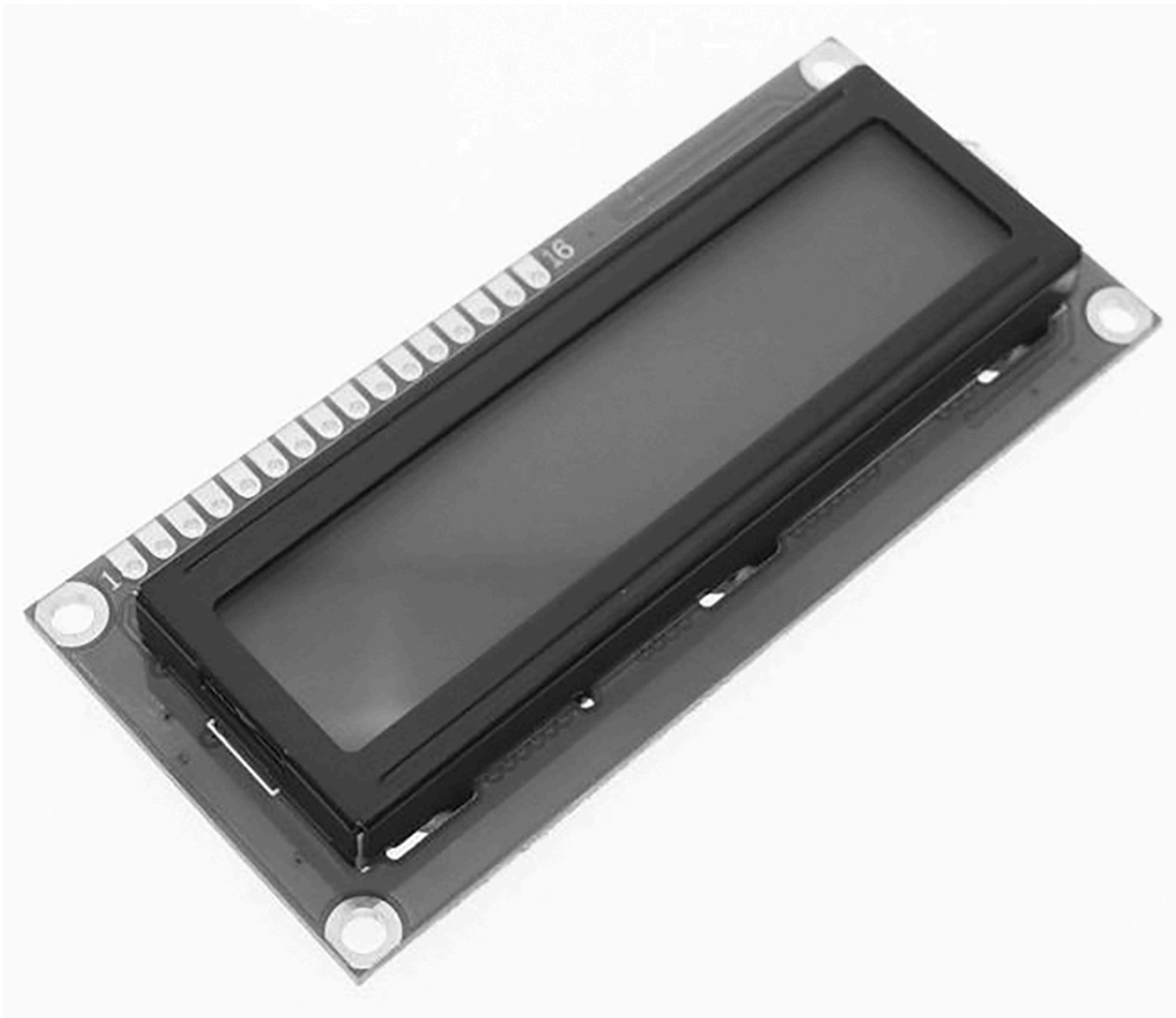
Figure 13-1: A 16×2-character LCD module
