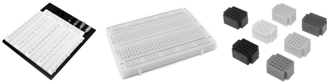
Figure 1-29: Breadboards in various shapes and sizes
