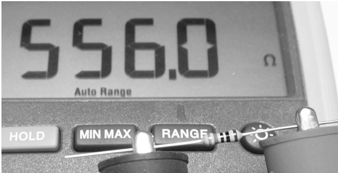
Figure 1-18: A multimeter measuring a 560 \Omega 1 percent tolerance resistor
