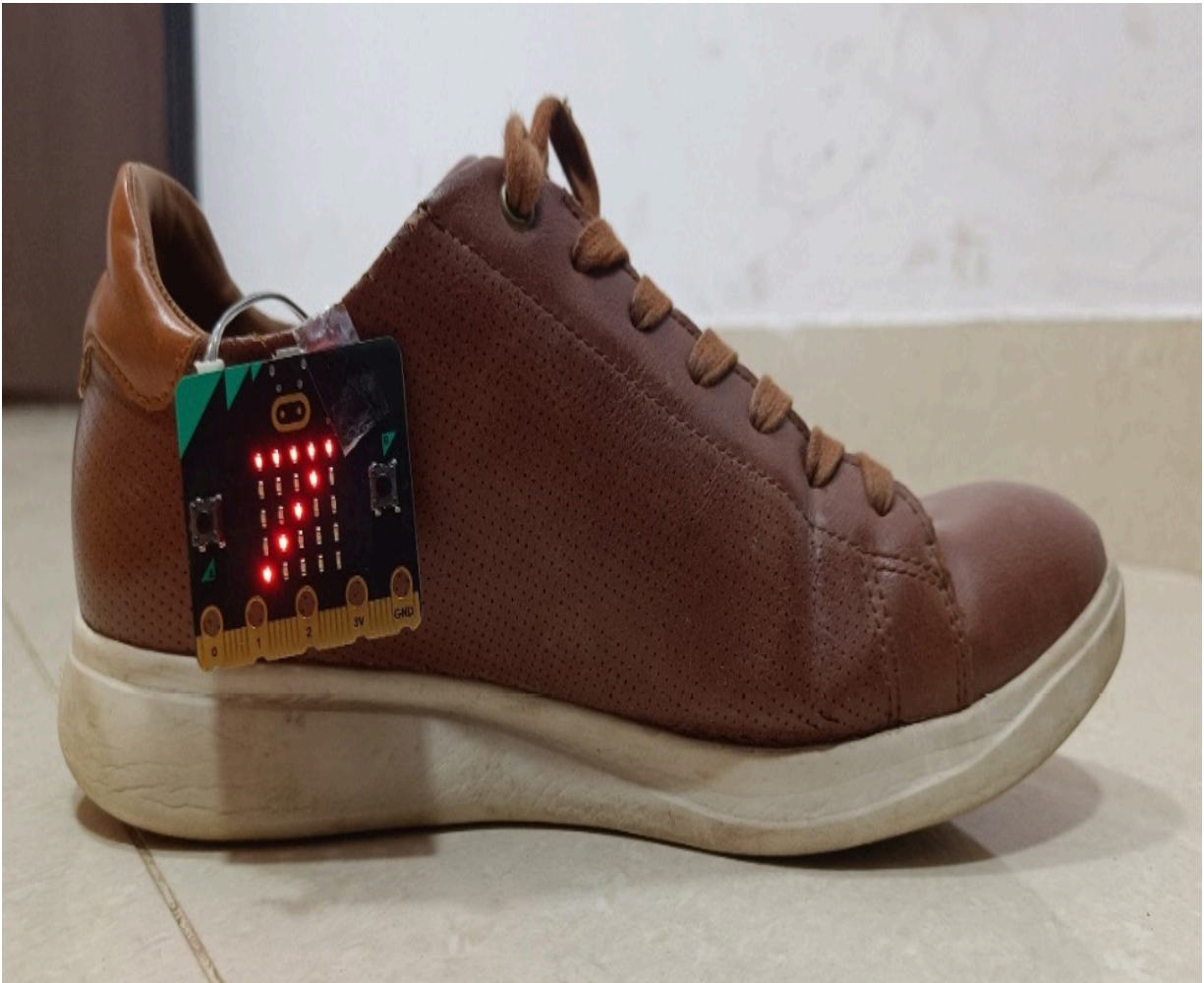
Figure 15.1 – A Micro:bit mounted on a shoe to count the number of steps the user takes
