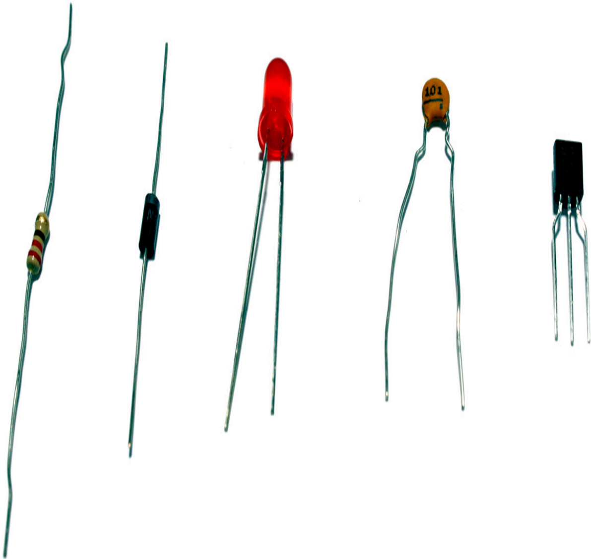
Figure 1.3 – Electronic components (shown from left to right): a resistor, a diode, an LED, a monolithic capacitor, and a transistor
