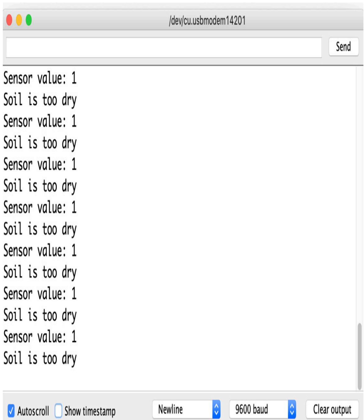
Figure 10.6 – Serial monitor readings with dry soil
