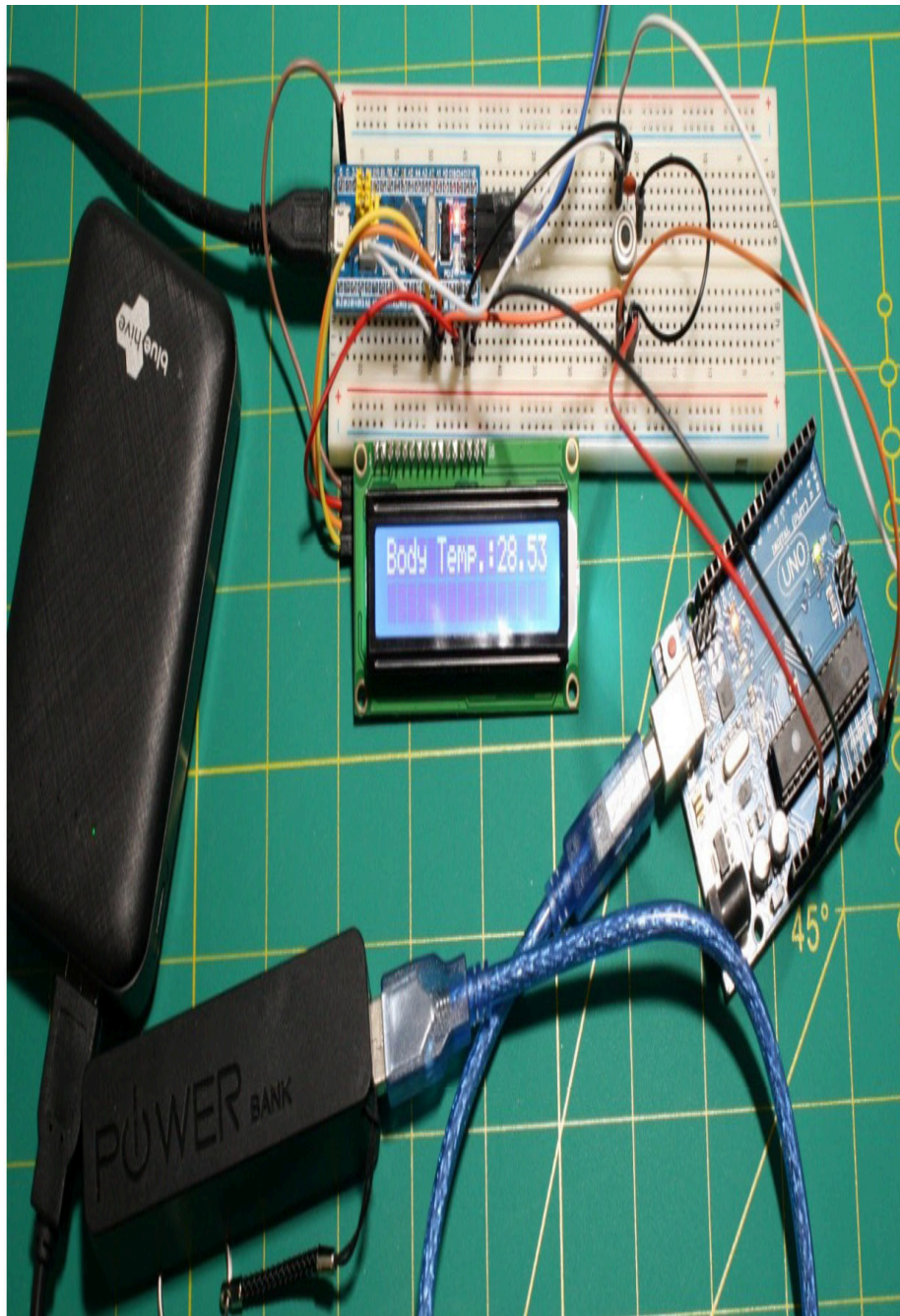
Figure 12.10 – The microcontroller boards, the sensor, and the LCD
