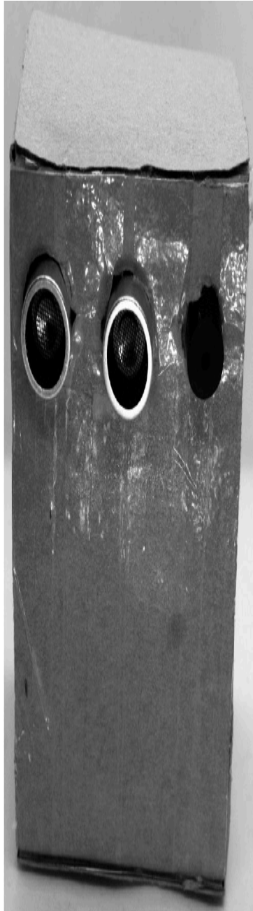
Figure 13.12 – A cardboard-case template for our device
