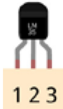
Figure 5.8 – The LM35 sensor showing pins 1, 2, and 3
