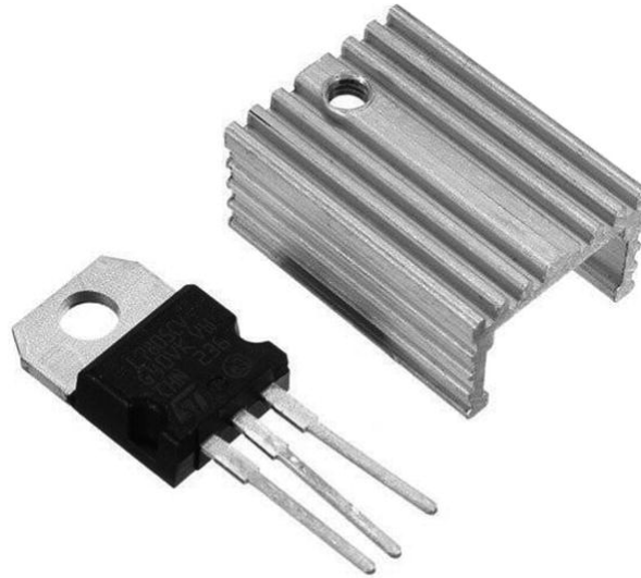
Figure 10-1 A 7805 voltage regulator and its heatsink
