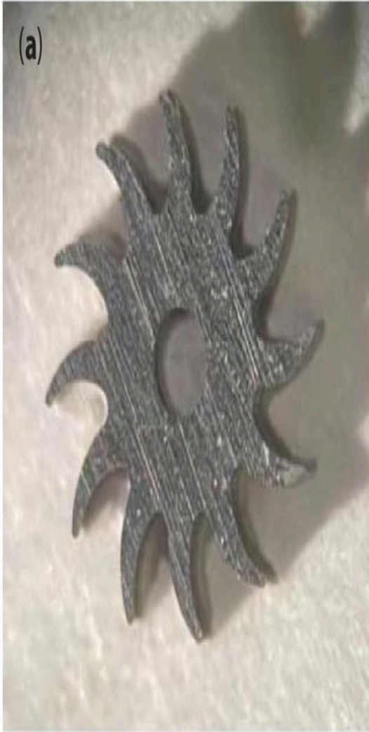
Figure 11.26 Fabricated two type shape rotor (a) sharp design (b) blunt angle design.
