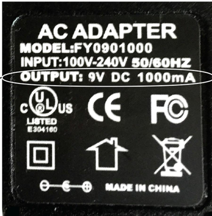
output of this supply is 1000 milliamps, or 1 amp, and 9 volts DC
