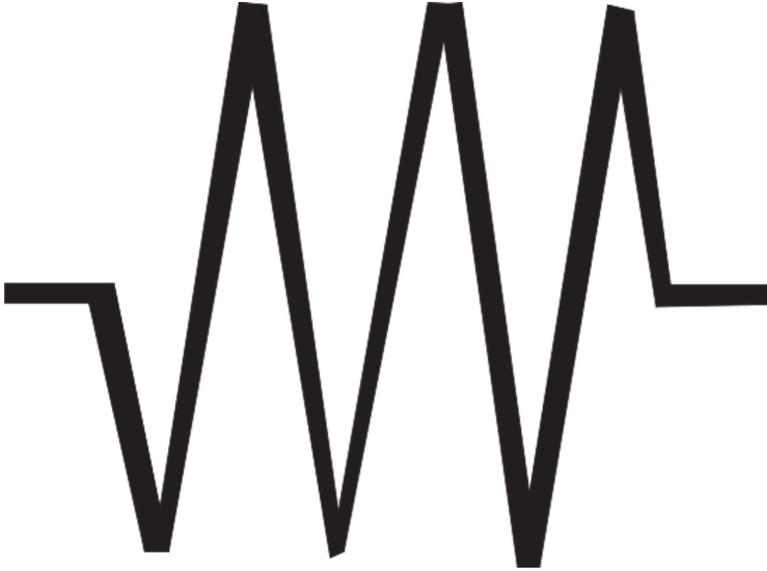
**FIGURE 3-12:** Schematic symbol for a resistor
