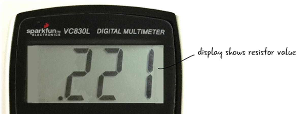
**FIGURE 5-33:** Multimeter display showing resistance value
