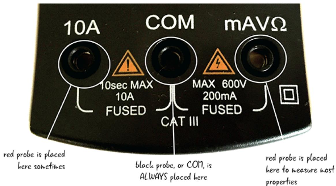
**FIGURE 3-40:** The ports on a multimeter
