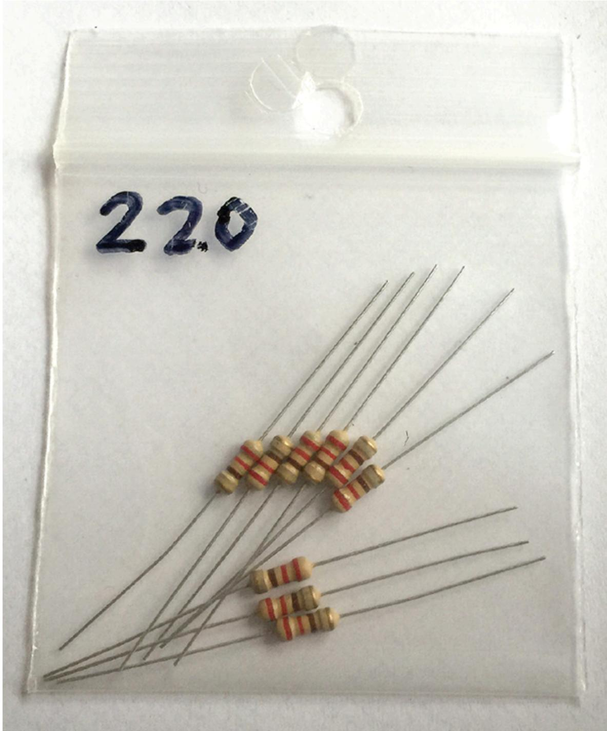
**FIGURE 5-30:** A package of resistors
