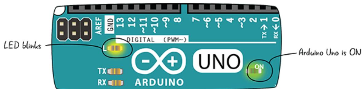
**FIGURE 4-12:** Indicator LEDs
