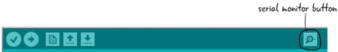
**FIGURE 7-24:** Serial monitor button
