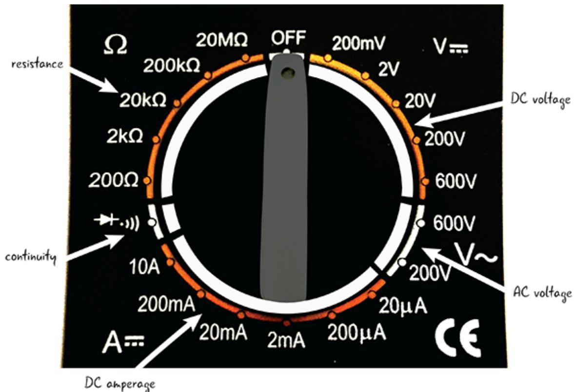
**FIGURE 3-38:** The dial of a multimeter with electrical properties it can measure
