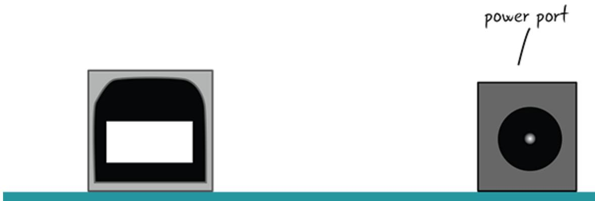
**FIGURE 2-9:** Power port on the Arduino
