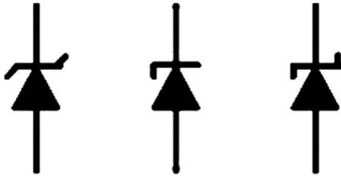
Figure 3-20 Zener diode schematic
