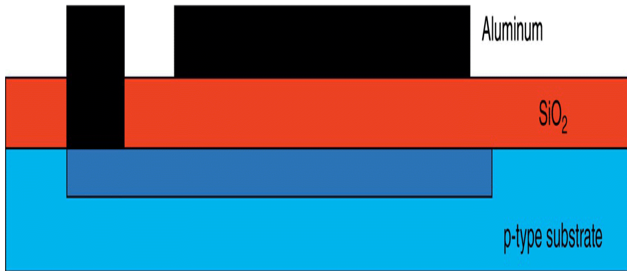
Figure 10.22 Capacitors are fabricated using the same techniques as MOSFETs with a heavy doped semiconductor and a metal plate separated by the SiO 2 insulator.
