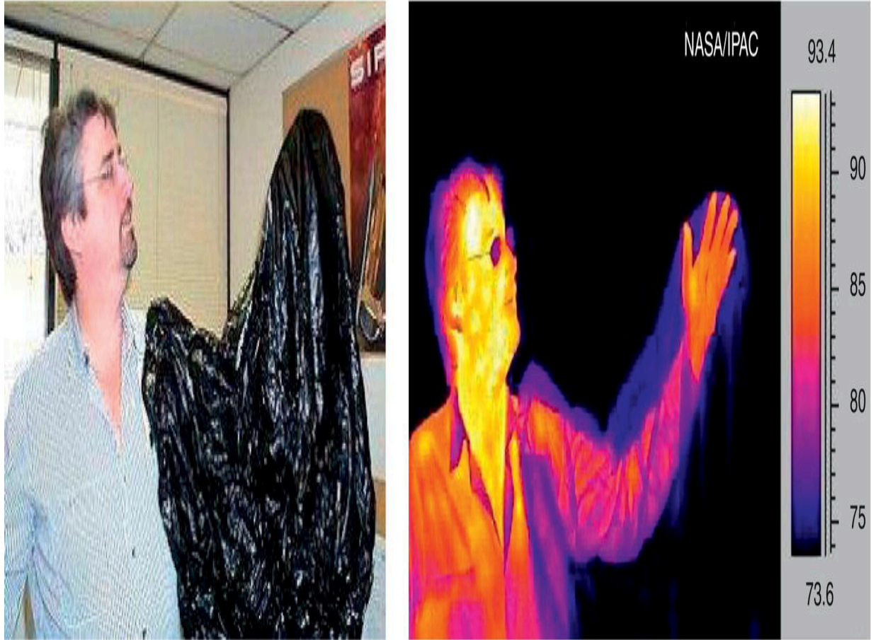
Figure 4.7 On the right the man hides his arm with a plastic bag. The arm is fully visible in the infrared photograph on the left.
