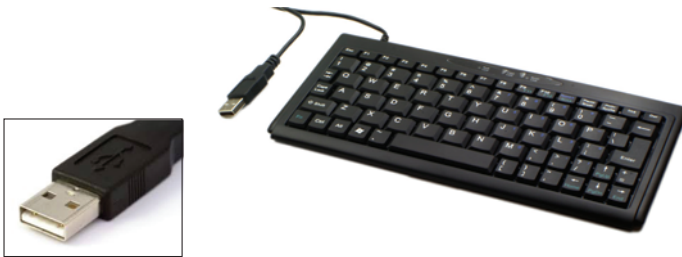
Figure 1.5 You need a USB keyboard to type and enter commands on your Raspberry Pi. The keyboard plugs into one of the four available USB ports on the Raspberry Pi 2 Model B.
