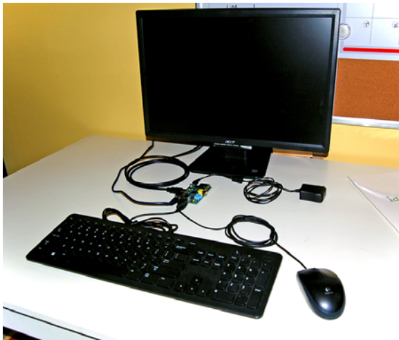
Figure 1.12 Example setup of a Raspberry Pi with peripherals connected and SD card inserted. A keyboard and mouse are connected to the Pi's two available USB ports. A microUSB power supply is plugged into the Pi; the other end is lying on the desk, ready to be plugged into the wall. An HDMI cable is connected from the Pi's HDMI port to the back of the monitor. The Ethernet port has an Ethernet cable plugged into it from a router (not shown).
