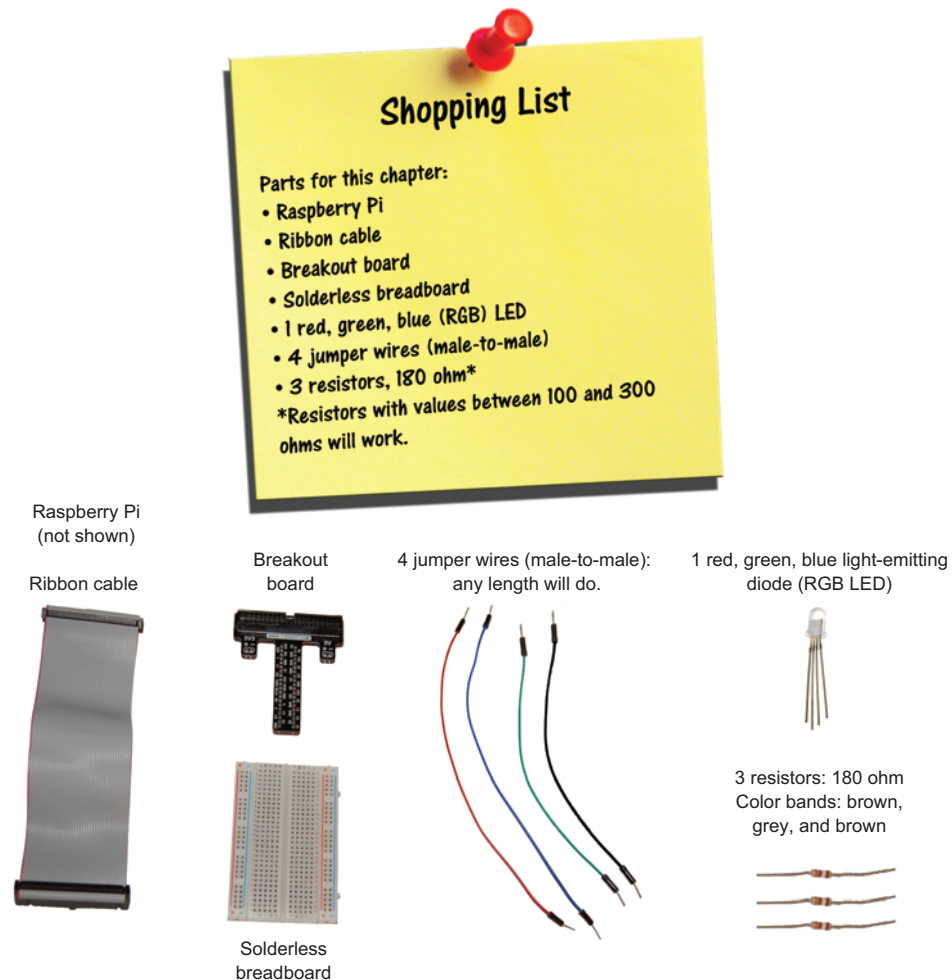
Figure 7.1 The Light Up Guessing Game uses a red, green, blue (RGB) LED. An RGB LED can produce many different colors because it has three LEDs (colored red, green, and blue) packed inside it.
