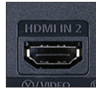
Figure 1.8 HDMI and DVI are common types of video input ports found on modern TVs and monitors. It's easiest to connect a Raspberry Pi to a TV or monitor with an HDMI port. HDMI provides a high-definition picture and doesn't require any adapters or converters—only an HDMI cable, which is included in many Pi kits. The DVI port requires a special adapter to connect with a Pi.
