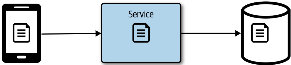
Figure 4-14. Client uploading a file that's passed through the service
