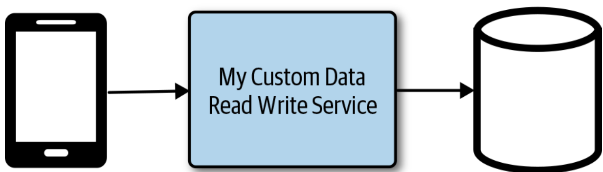
Figure 4-13. Client application with a backend service and database
