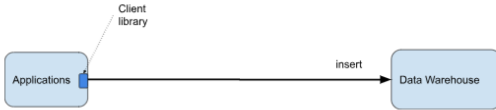
Figure 9-4. Streaming ELT in a cloud-native application can take advantage of client libraries to directly insert the data.
