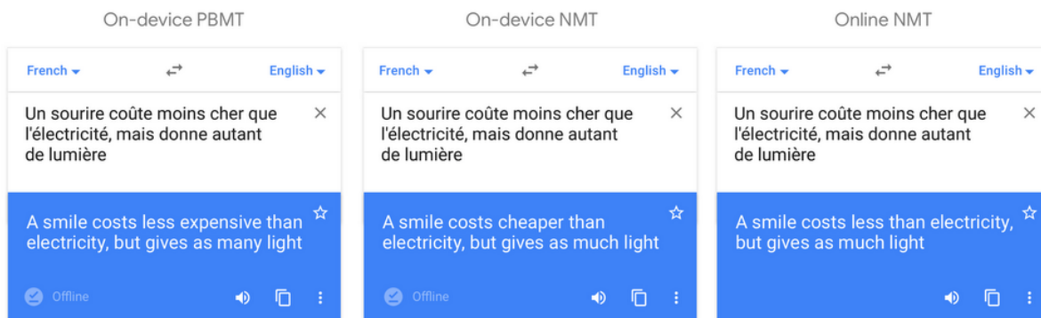
Figure 5-12. A comparison of on-device phrase-based and (newer) neural-machine translation models and online neural machine translation (source: The Keyword ).
