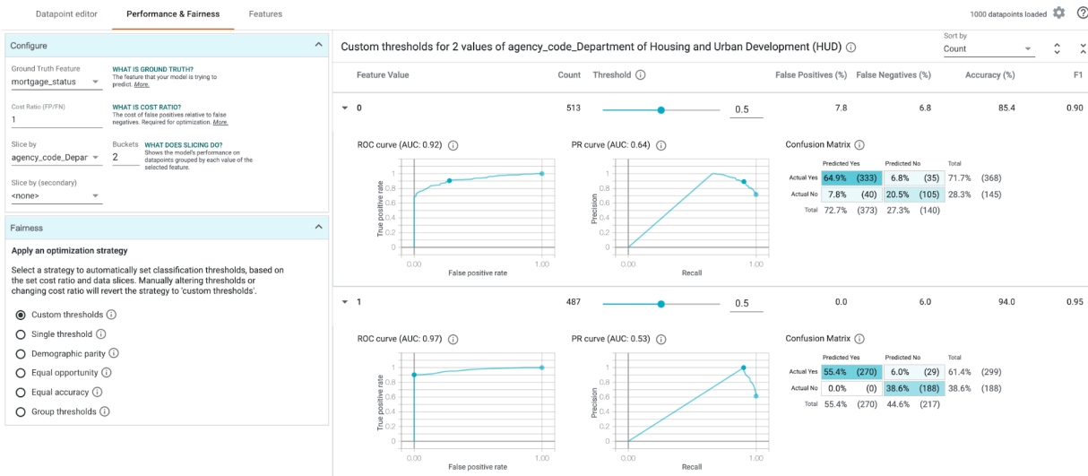
Figure 7-14. The What-If Tool Performance & Fairness tab, showing our XGBoost model performance across different feature values.
