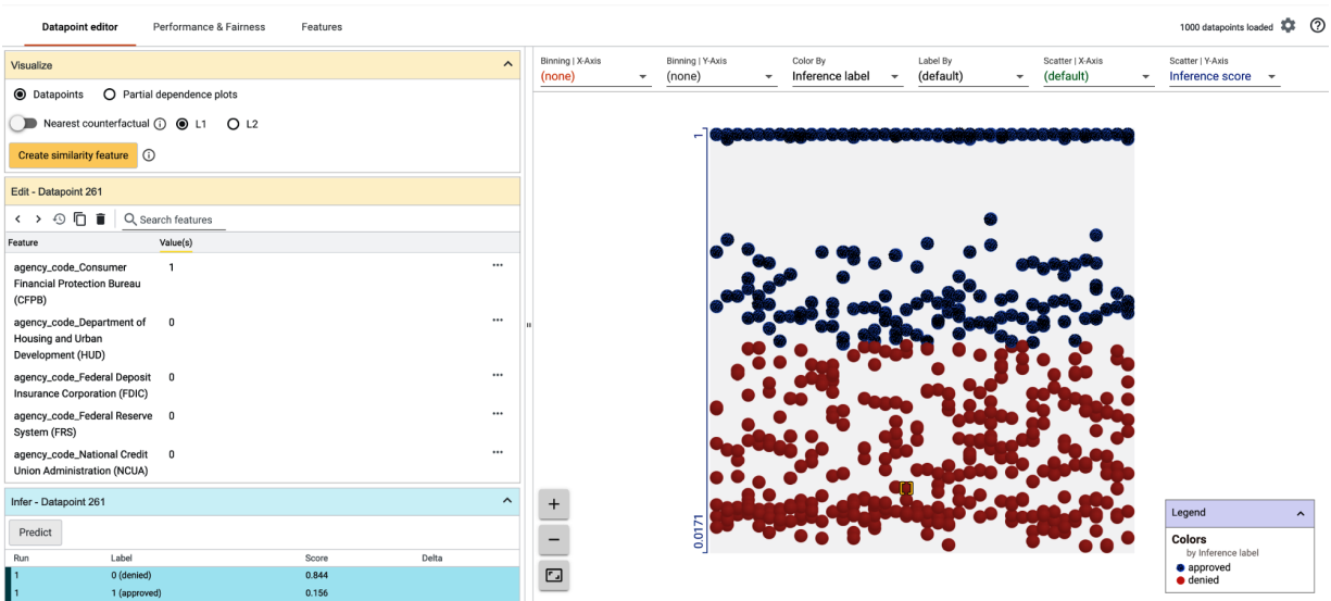
Figure 7-13. The What-If Tool's Datapoint editor for a binary classification model. The y-axis is the model's prediction output for each datapoint, ranging from 0 (denied) to 1 (approved).
