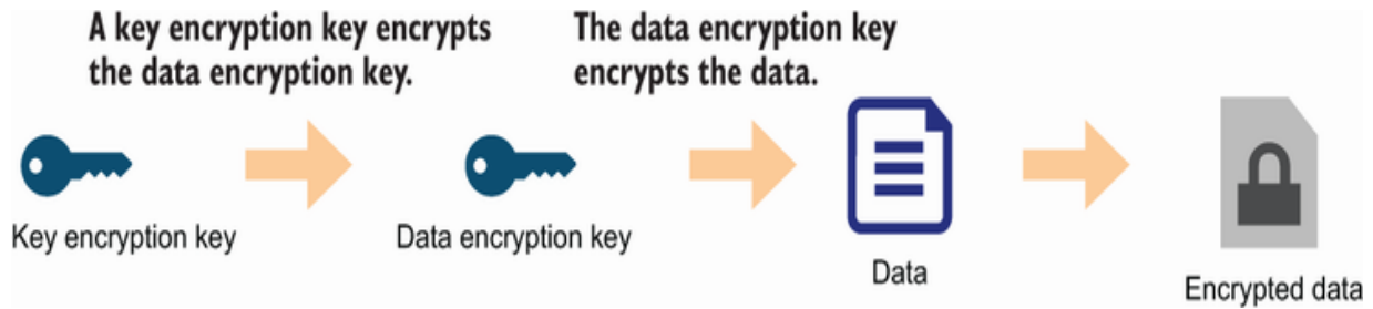
Figure 14.11 Envelope encryption is the practice of encrypting data with a data encryption key (DEK) and encrypting the DEK with a key encryption key.
