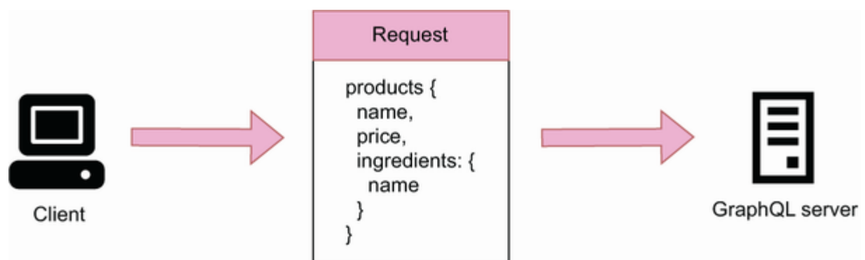
Figure A.8 Using a GraphQL API, we can query data from related entities, such as products and ingredients. In this figure, an API client requests a list of products with the names of their ingredients.
