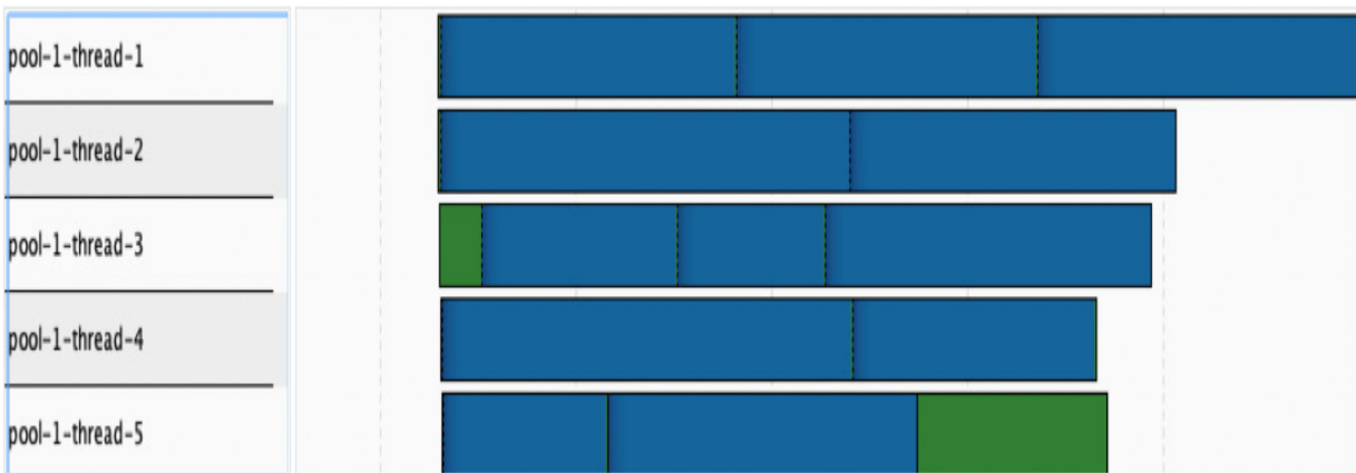
Figure 6.17 – The behavior of the thread pool shows the usage of the created thread
