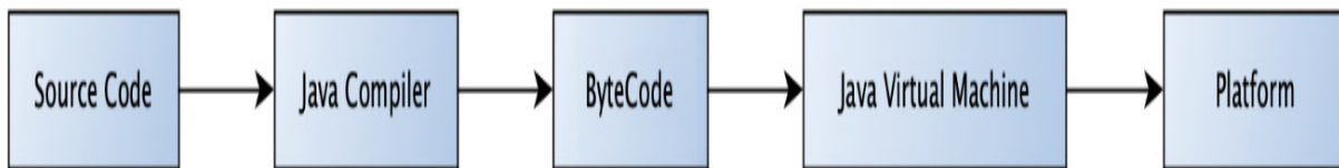
Figure 1.3 – A simplified flow for the Java program through the compiler to its platform execution
