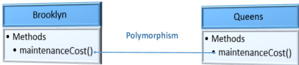
Figure 2.11 – Polymorphism of one method in independent classes
