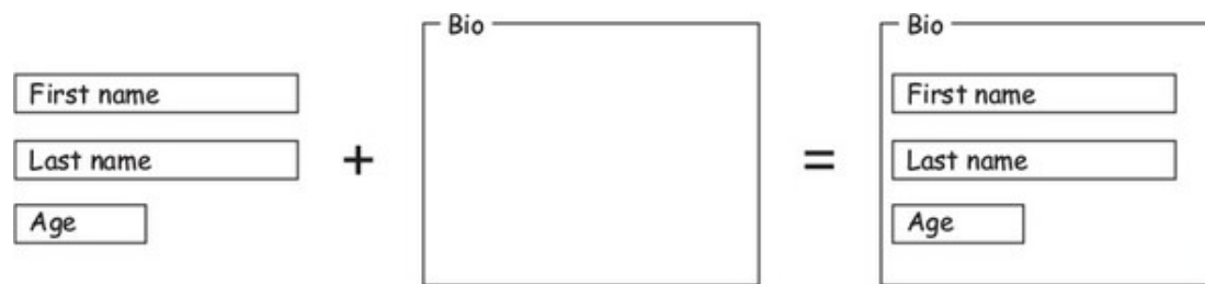
Figure 4.7. Combining three simple input text widgets with a container widget to create a bio form component
