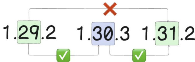
Figure 19-2 Kubernetes supported version upgrade process
