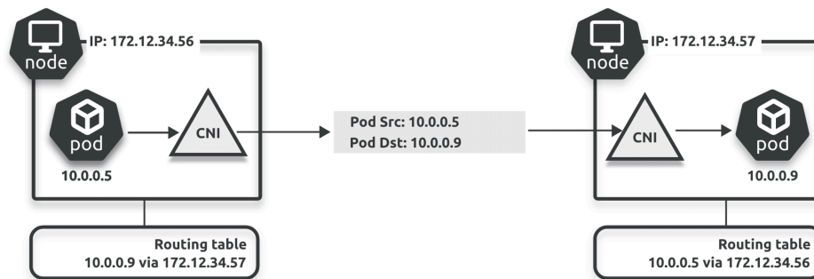
Figure 17.6 - No encapsulation on BGP network
