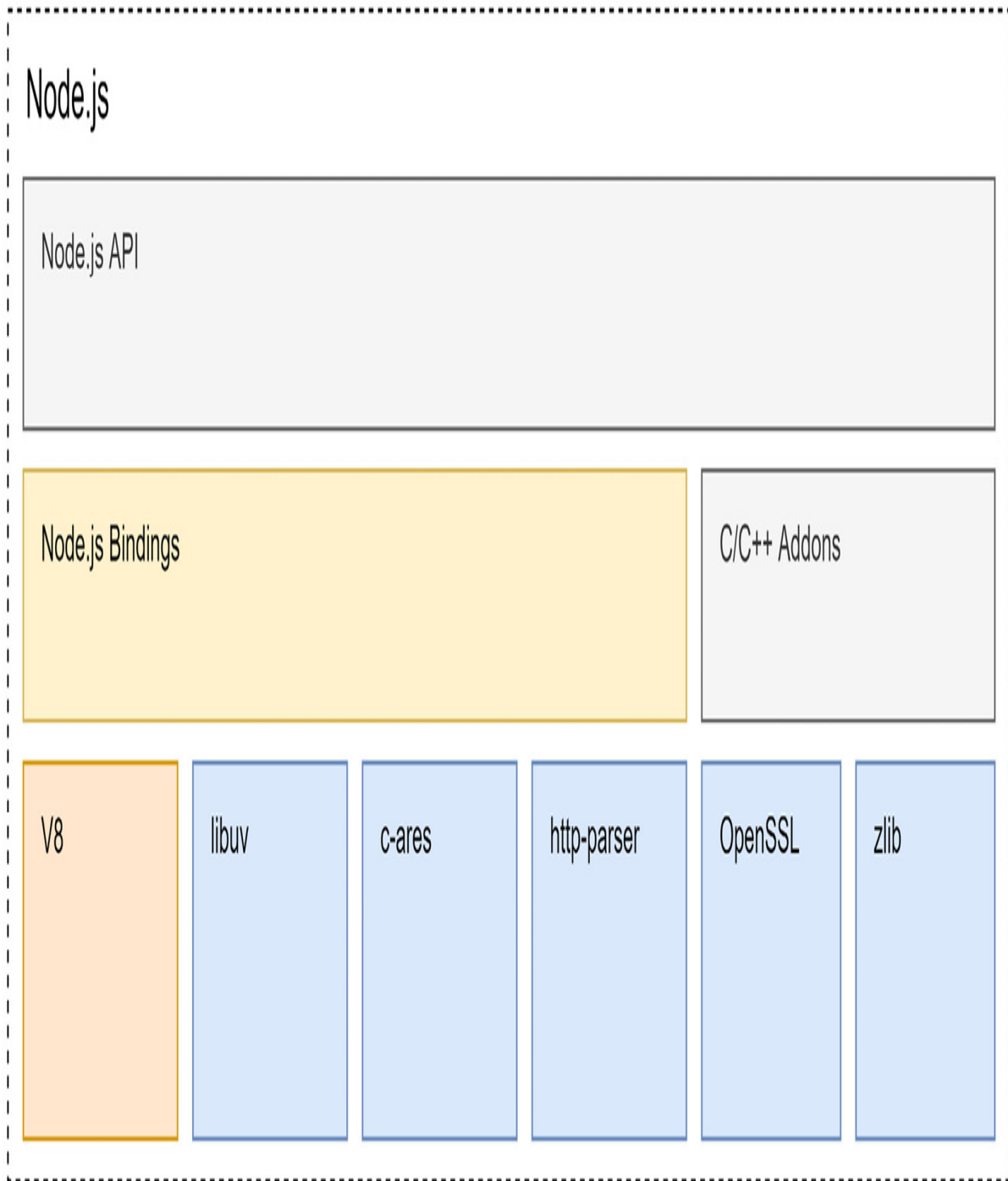
Figure 1.2 – Composition of Node.js in terms of building blocks
