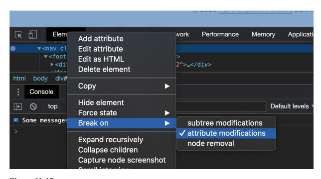
Figure 11-17 Setting up a break element on attribute modification
