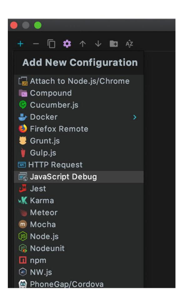
Figure 11-4 Add New Configuration window for JavaScript debugging
