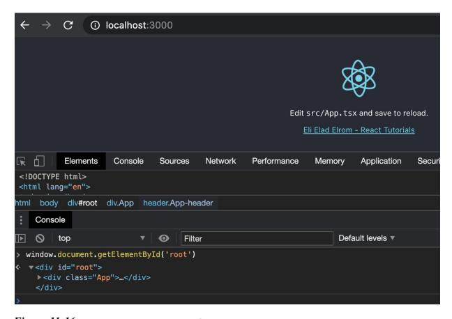
Figure 11-16 Inspecting the root element in Chrome DevTools
