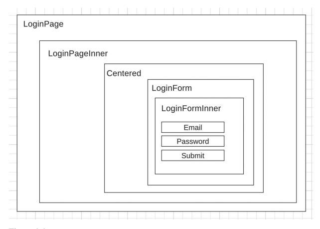
Figure 6-6 LoginPage component and subcomponents
