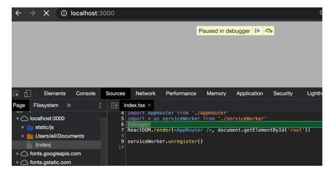
Figure 11-8 Stopping the rendering of the Chrome browser using the debugger statement
