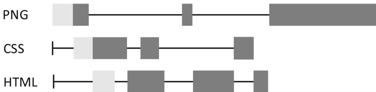
Figure 5-10 Multiplexing in HTTP/2
