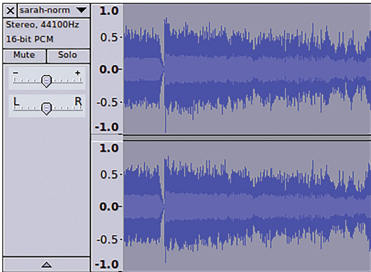
Figure 8-3 Audacity confirms that the volume has been increased without cutting into the waveform
