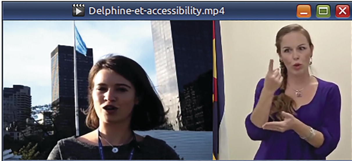
Figure 7-2 The scale filter was used to reduce the height of the first video. The pad filter has been used to expand the frame of the scaled video. The overlay filter has been used to place the second video in the empty area of the expanded frame
