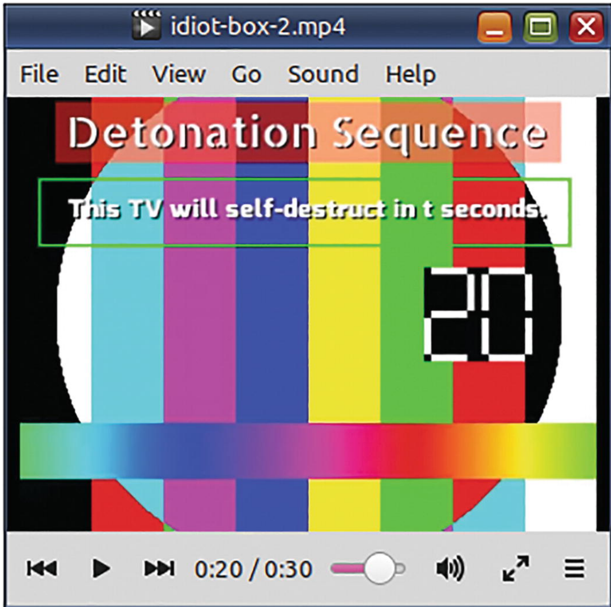
Figure 7-16 With the drawbox filter, two rectangles around the text. (See original video in previous section.) The first rectangle is filled with red. The second rectangle is bordered green
