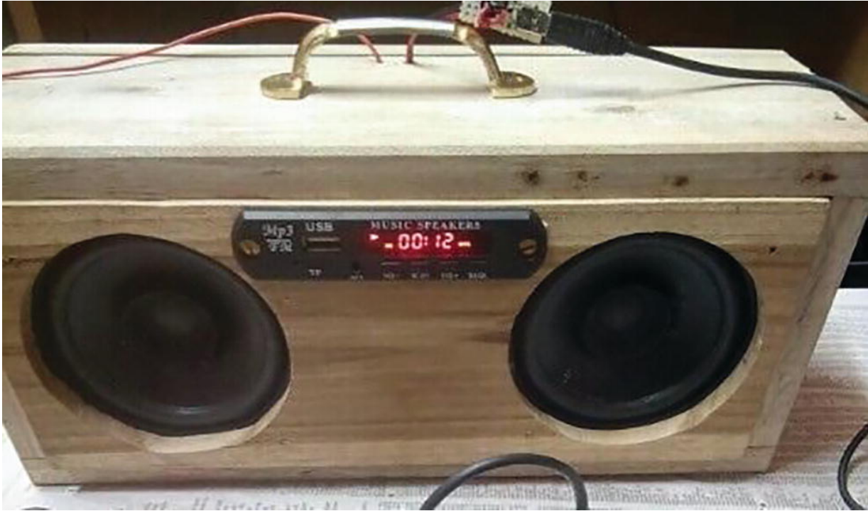
Figure 11-5 I built this boombox. The MP3 player module's display is limited to song numbers
