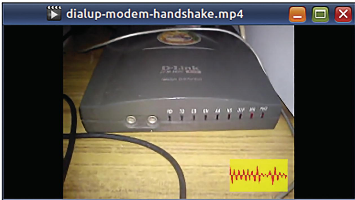
Figure 8-7 This command draws a waveform of the dialup modem handshake tones on the video. To make the waveform easily visible, the command has drawn a translucent yellow box behind it
