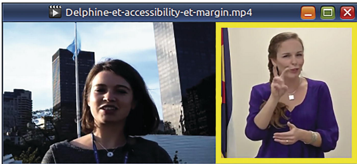
Figure 7-3 The pad filter was used to expand the width of original frame by 360 pixels while maintaining the same height. The expanded area was given a yellow background that was 360×360 pixels. Using filter expressions with the overlay filter, the 332×332-pixel second video was placed right in the middle of the yellow background
