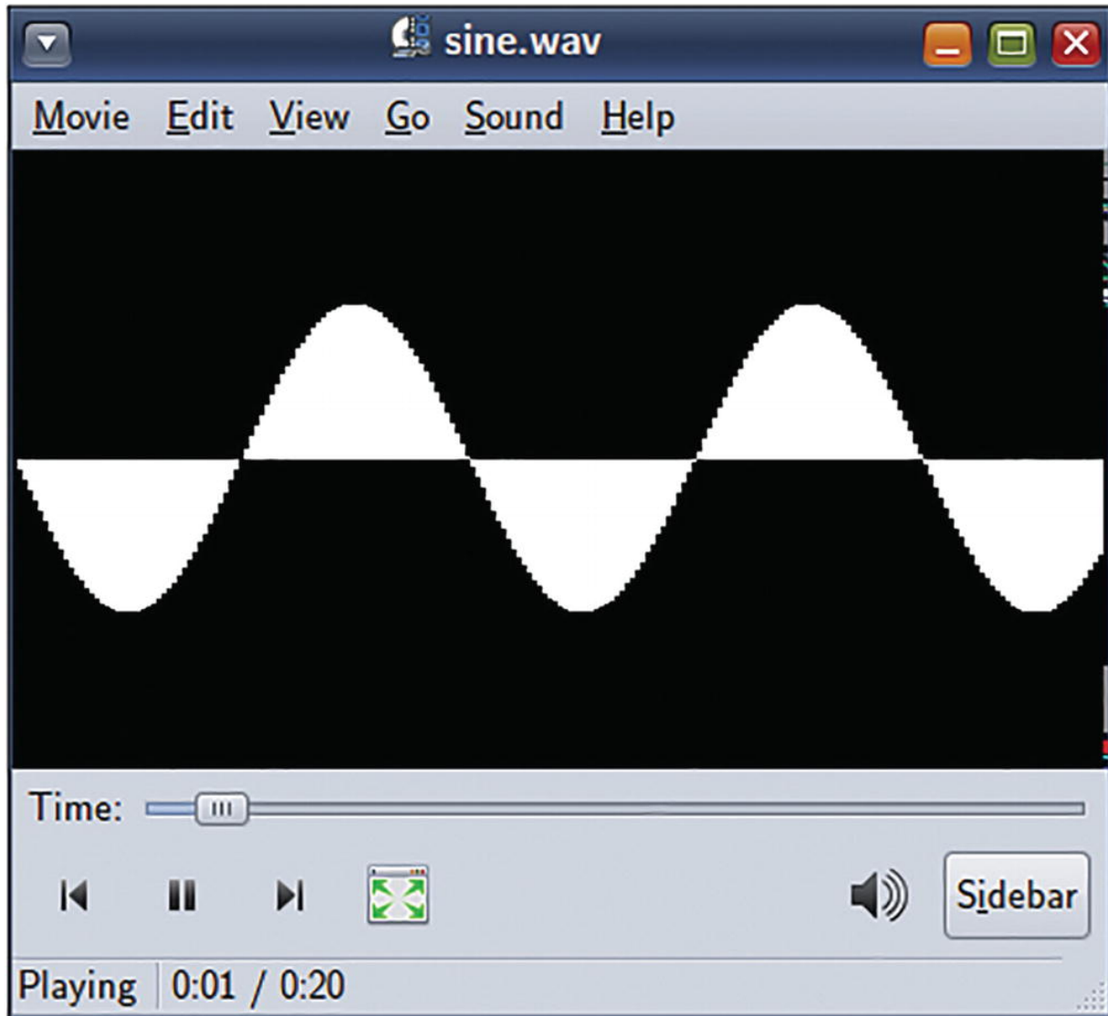
Figure 11-14 The visualization feature of this media player confirms that the audio is a sine wave
