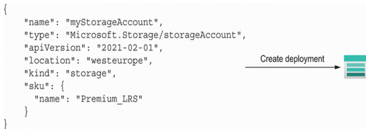
Figure 1.1 From ARM template to Azure infrastructure
