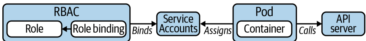
Figure 3-2. Using a Service Account to communicate with an API server
