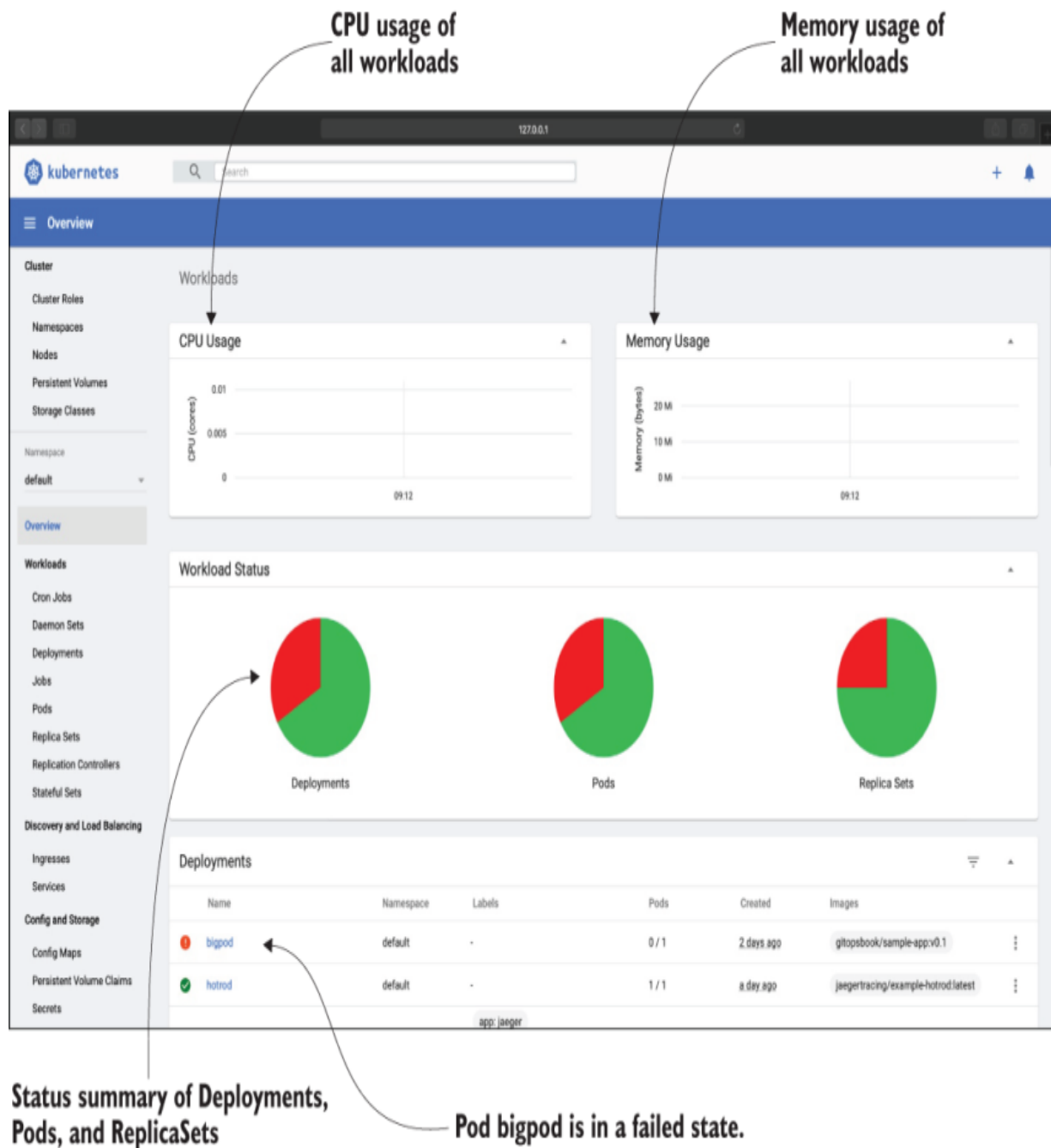
Figure 8.9 The Overview page of the Kubernetes Dashboard shows the CPU and memory usages of the workloads currently running on the cluster, along with a summary chart of each type of workload (Deployments, Pods, and ReplicaSets). The page's bottom-right pane
